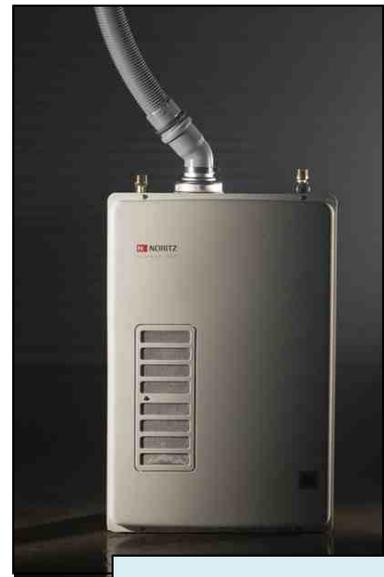
The Noritz EZTR40 with top-mounted water connections and two-inch, flexible polypropylene tubing for threading directly through existing B-Vent, dramatically reducing installation time.
